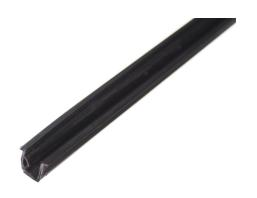
A plastic profile / seal that fits in series 30 and 40 profiles with 8mm slots. t can hold a 5mm plate inside the slot, for example for making covers and shields.
