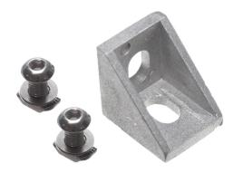
A bracket in aluminium for joining two series 20 profiles in 90 degrees. There are knobs under the brackets to keep them in the slot while tightened. The knobs can also easily be ground down, if you need to mount the brackets transversal.
