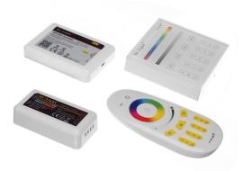
RGB+White system for 12V and 24V products, such as LED strips. Color and effect can be controlled with various units - remote, touch control panel and also the wifi bridge for smart phones. Receiving distance maximum 30 meter. The controller can supply max 6A per color channel, or total 12A.
