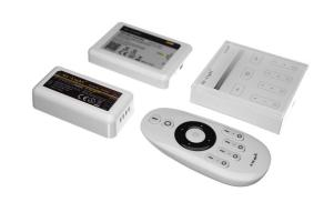
A light dimmer for 12V and 24V such as LED strips, that is easily controlled wireless with a remote, touchpanel or a wifi bridge so it can be controlled with your smartphone using an app. The controller has 2 output where each can draw up to 6A, total A is however max 12A. The receiving distance is maximum 30 meter.
