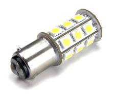
BAY15D LEd bulb for 6V~9V vehicles with 2 light outputs corresponding to 21/5W. The bulb is + controlled and it only works on vehicles were the taillight and breaklight are activated by a + wire. This only works on DC / direct current.
