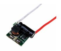
An unprotected mini LED driver to provide a high power LED with the right amount of power.
