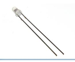
3 mm diodes with integrated resistance, which means that you can connect 12V directly to the diode without a dropping resistor. 60 degree dispersion angle. It is suitable to build it in contacts etc., where the bulbs cannot be swapped out with a diode bulb.
