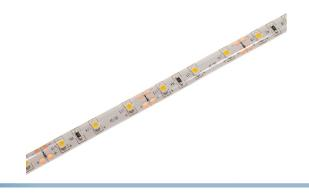
The splashproof LED Tape SMD can be shortened or extended further, so it fits for your project. The stripe is 8/10 mm wide and is built up in small modules of 5 cm or 10 cm, where there are 3-6 heavy SMD diodes in a circuit ready for 12Vdc. There are clear markers where the stripe can be cut, as well as solder-islands, where you can solder wire on or extend with more SMD-tape. On the back is a 3 m powerful tape, which makes that LED SMD tape to stay attached to his seat without screws.
