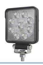
E-Approved working lamp with 9 powerful Osram LEDs. Alu-house with powder-coating and stainless steel bracket. The light color is 6000K and lens of 60 degrees gives a good diffusion of light, suitable for work.
