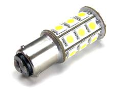
An extra heavy BAZ15D Xenon White LED bulb with 24 pcs. 5050 SMD diodes, which together make 270 lumens. The LED bulbs are used for the run/position lights. The LEDs bulb location makes the whole dish to light up. The bulb has a built-in voltage regulator that protects from overvoltage and thereby also provides a longer life.
