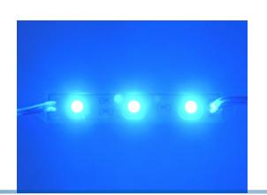
Splash-proof LED modules, which can be used for example as a signal lighting.
