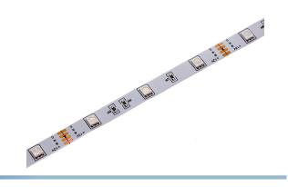
LED SMD stripe can be shortened or extended further, so it just fit for your project. The stripe is built up in small modules of 10 cm, where there are 3 powerful SMD diodes in a circuit ready for 12Vdc. There are clear markers, where the stripe can be cut, as well as solder-Islands, "where you can solder a wire on or extend with more SMD stripe. On the back, there is a powerful 3 m tape, which makes the LED SMD stripe to stary attached without screws.
