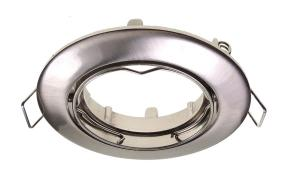
A beautiful swivel MR16 downlight in a brushed steel. An easy fitting by making a hole of 73 mm, after which the downlight springs push back and the downlight is pressed into the hole.
