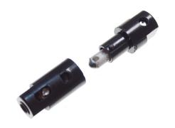
Simple fuseholder with screwterminals, that use the small Bosch / GBC fuses. 8A fuse included. Wires are easily mounted in both ends using the screw terminals.
