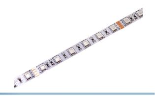
LED stripes can be shortened or extended further so it just fit for your project. The stripe is 12 mm wide and built up in small modules of 10 cm where there are 6 powerful SMD LEDs in a circuit ready to 24Vdc. There are clear markers where the Ribbon can be cut, as well as solder-Islands "where you can solder wire on or extend with more LED stripe. On the back is a powerful 3 m tape which ensures that the LED stripe stays attached without screws.
