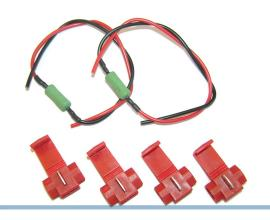
When switching from 5W position light bulbs to LED ones, the power consumption will get lower than usual and therefore might be experienced error messages on some newer cars with bulb-control. Because of this you will have to apply these "cheat light bulbs", which raise the consumption, so that it matches a regular bulb. The resistors will be connected to the + and - approach to the socket/bulb.
