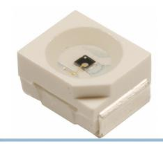
110mcd 120 \* - suitable for instrument lighting in VW from year 97 and above
