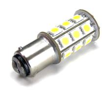
A warm white Ba15D marine LED bulb with 24 pcs. 5050 SMD diodes, which together make 280 lumen. The bulb may well replace a regular  $20 \sim 30$  watt incandescent bulb and the natural color makes the bulb suitable for lighting in the cabin/stateroom/Lantern.
