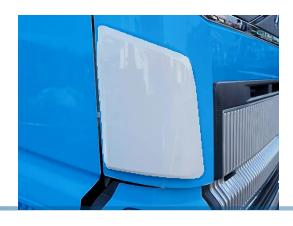
Dirt deflectors for Volvo FH5 with a custom-made design. All the mounting screws are hidden on the backside of the deflector and is very easy to mount.
