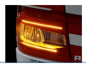
Adapter for the LED headlight on Scania +2016, that turns on yellow position lights in the top indicator at low brightness, and full when indicating.
