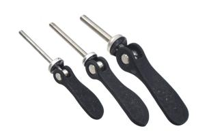
Cam lever with thread bolt, that can be used to fasten / lock parts. Often used when you need to be able to easily change or adjust a setup without tools. Often seen used on bike seats etc.
