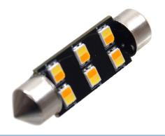
Bright Dual Color festoon bulb, with a total of 6 dual color LEDs. Changes color when polarity is flipped. This is either done with a 2-pole switch, or with one of our polarity flippers or color-changing controllers.
