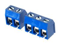
Screw terminals for through hole mounting in PCBs. 5mm pitch, 0.6mm pins. Available with 2 and 3 positions, that can be connected in a longer row.
