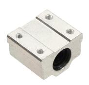
Linear block for 8mm axle, with holes for mounting of part, typically called SC8UU. There are 4 rows of balls inside the block, which gives you an even and precise movement.
