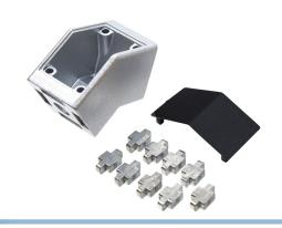
Bracket for joining two series 30 profiles in a 45 degree angle. You cut thread (M8) in the end of the profiles, and the bracket is bolted on to the ends. The small metal pieces are put in to the bracket, where they go in to the profile, and prevent the bracket to be twisted / rotated.
