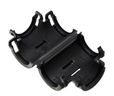
Splitter that fits NW17 corrugated tubes. Easy joining with click-locks. The three tubes are put in to the splitter, then it is foldes until the locks engage.
