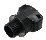
Gland for NW17 tubes, with M20 thread. The tube is pushed in and locks itself. The gland is fastened with a M20 nut.
