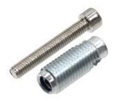
Screwed in to the end of a track on a series 40 profile, where after the included bolt is put through and used for fastening, eg. with a sliding nut or spring nut.
