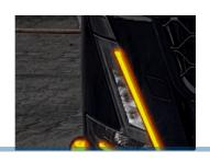
Complete set LED emitters for retrofitting your Volvo FH5 or FM5 with amber DRL, or simply for replacing your emitters if one of the original breaks. These fit Volvo FH5 and FM5 from 2021 and forward. There are in total 8 high-power LEDs per set with an output that is equivalent to the original.
