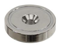
Magnets that can be fastened with countersunk bolts and screws. The countersunk hole gives you a flush surface after mounting. The magnet can be used for many purposes, eg. as a tool holder.
