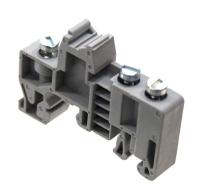
End-stop for DIN-rails. Clicked on and fastened with the 2 screws. Prevents the other elements from sliding on the rail.
